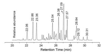
Fig. 6. GC-MS spectrum of the C12 dimers (measured by GC-MS with DB-5MS column, Cat. 4a  $7 \times 10^{-5}$  mol, MAO 80 mg, temperature 45 °C, 3h)
