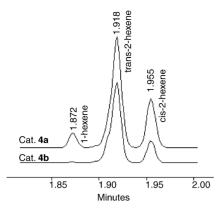
Fig. 3. GC spectrum of the hexene isomers (measured by GC with HP-5MS GC column, 1-hexene 0.01 mL, Cat. **4a** and **4b** =  $7 \times 10^{-5}$  mol, MAO 80 mg, temperature 45 °C, 3 h).
