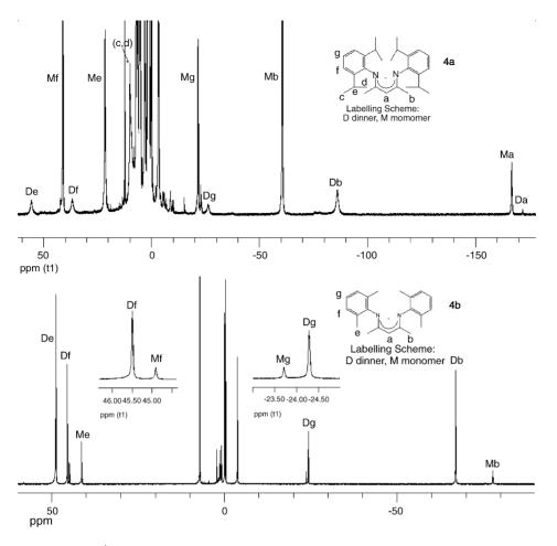
Fig. 2. <sup>1</sup>H NMR spectrum of complex 4a and 4b in C6D6 ( $\sim$ 10 mmol/0.5 mL), at 30 °C.
